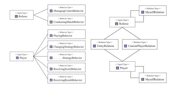
Fig. 9. Class diagram of the extended IPD model
